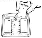
4. Insert 3 C-Cell batteries.
