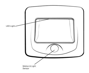
NOTE: Light sensor only allows light to activate in darkness. We recommend you test in a dark room or closet.
