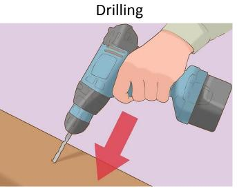
Hold the drill steady and apply consistent pressure into the project panel
