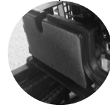
AIR FILTER (AIR FILTER COVER HAS BEEN REMOVED)
