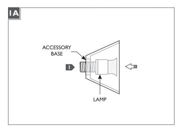
**CAUTION:** To reduce the risk of a burn or electric shock during relamping, disconnect the power to the fixture.
