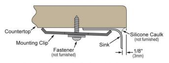
Designed to affix to the underside of any solid surface countertop.
