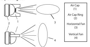
Trigger a short burst while turning the fluid control knob counterclockwise. Observe the spray pattern on the target and adjust the fluid control knob until the desired atomization is achieved.
