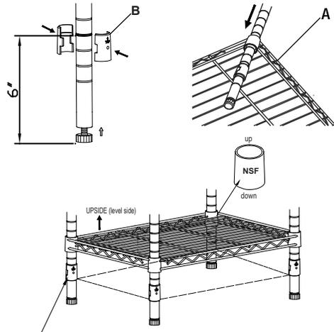
Note: The tapered sleeves must be at the same height for each pole to ensure the shelf sit on the sleeves levelly.
