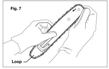
7. Hold the chain in position on the bar and place the loop around the sprocket. Fit the bar flush against the mounting surface so that the bar stud is in the long slot of the bar and the adjusting pin is in the chain tension pin hole (Fig. 8)
