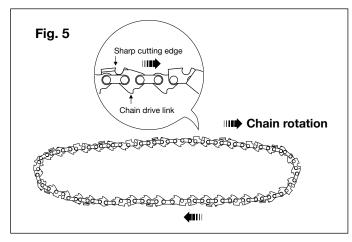
**6.** Starting at the tip, mount the chain drive links into the bar groove, leaving a loop at the back of the bar. The chain will loosely fit until it is placed on the sprocket. (Figs. 6 & 7)
