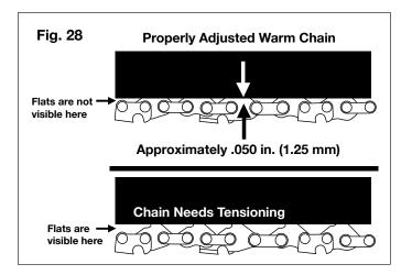
**NOTE:** A new chain tends to stretch. Check the chain tension frequently and re-tension as needed.
