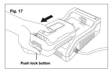
**8.** Timely recharging of the battery will help prolong the battery's life. You must recharge the battery pack when you notice a drop in the equipment's power.
