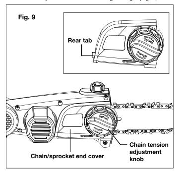
9. Turn the ring nut clockwise until you find the right chain tension, then tighten the chain tension adjustment knob securely (Fig. 10).
