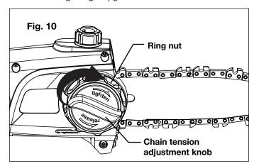
**NOTE:** If the chain is too tight, it will not rotate. Loosen the chain tension adjustment knob slightly and turn the ring nut 1/4 turn counterclockwise. Lift the tip of the guide bar up and retighten the chain tension adjustment knob. Ensure that the chain can be rotated by hand without binding (Fig. 11).
