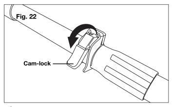
**AWARNING!** Failure to lock the telescopic pole cam-lock as directed could result in personal injury.
