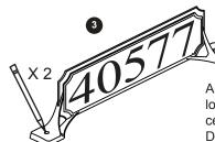
Align plaque at desired location and mark the center of each hole.
