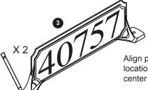
Align plaque at desired location and mark the center of each hole.
