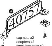
Place adapters into the feet of the plaque and secure with 2 small hex bolts and 2 caps nuts.
