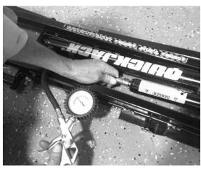
3. When the pressure is between 40 and 50 PSI, remove the pump or air compressor.
