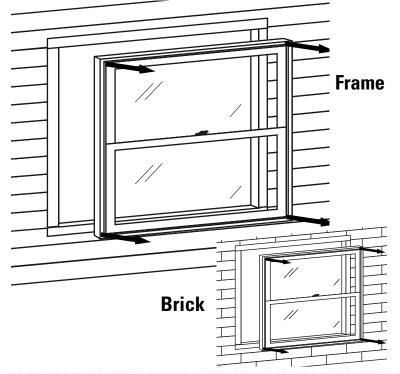
**SET UP.** Measure the existing opening (width & height) as if the existing window & frame were already removed from the opening. When choosing a replacement size window go down to the nearest even inch, both in width and height.
