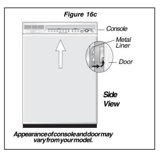
**6.** Unlatch door and open while supporting outer door on both sides at bottom to keep in place. Align screw holes and replace screws.
