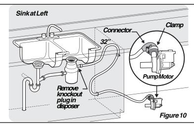
The drain hose loop must be at least 32" high from the floor to insure proper drainage.
