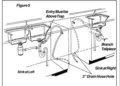
2. If you connect to a sink drain, entry will need to be above trap. A "Y" branch tailpiece and connector kit, not included, will make this method easier and includes all needed fittings and instructions. See Figure 5.
