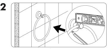
Level and mark position of the towel ring on the wall. **a.** If mounting into ceramic or tile, place masking tape on the mounting areas before marking the location to prevent the drill from slipping and damaging the tile.
