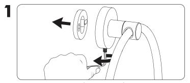
Remove mounting plate from back of towel ring. **a.** Use the provided allen wrench to loosen set screw on bottom of the towel ring to remove the mounting plate.
