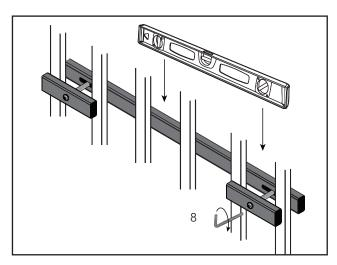
8. Level mounting rail and tighten snugly. Check for tight fit monthly.
