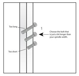
Determine bolt length by holding a bolt up to your spindles, a bolt that is about the same length or slightly longer than your spindle depth is the right one.
