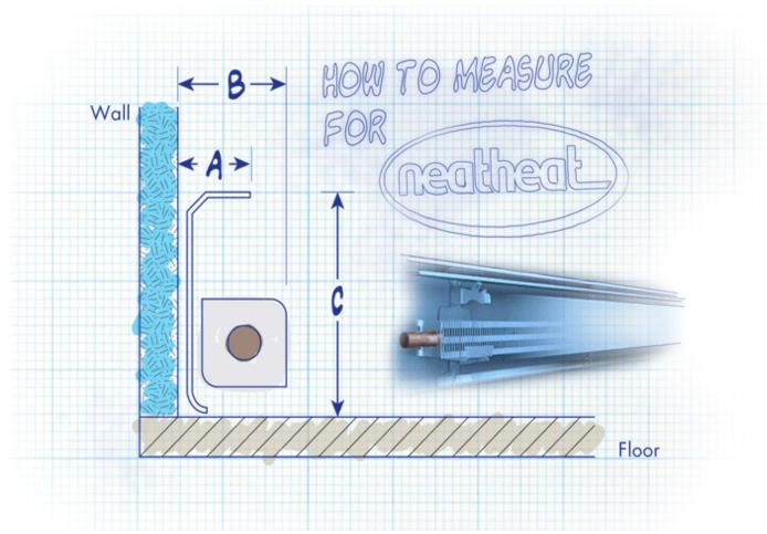
A = The measurement from the wall to the front edge of the metal enclosure attached to the wall. This measurement must be 2" or less.
