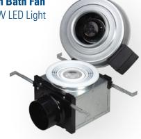
110 CFM fan, one ceiling grille with LED light, grille housing with a damper, dimmable 10W LED bulb. Uses 4" duct. ENERGY STAR® qualified. UL Listed for wet locations.
