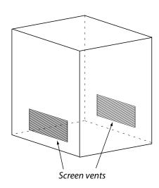
Make sure each opening has a total free area of not less then  $\frac{1}{2}$  square inch per pound (3.2 sq. cm/kg) of stored fuel capacity and not less then a total free area of 10 square inches (64.5 sq. cm).
