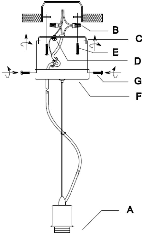
1. Attach the mounting bracket(C)to the outlet box by using two mounting screws(E).
