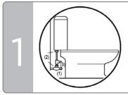
Shut water supply by turning it to the right and disassemble the water hose.
