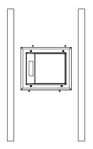
\*This product is designed for standard 2x4 framed walls. If your wall does not have the standard 3.5" spacing between the drywall you will need to use a kit that mounts on the front of the wall.
