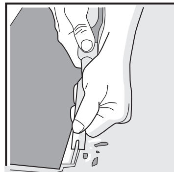
Fig 12. Horizontal installation (where angling is not possible). Cut off the locking element by using for example a chisel.
