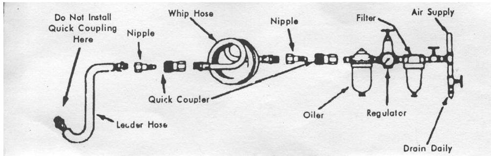
The air inlet, used for connecting air supply, has standard 1/4" NPT American Thread.
