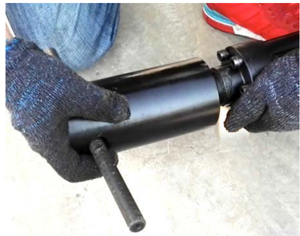
Fig. 6 ) Pull hard and wiggle Piling Socket Sleeve until it is removed.
