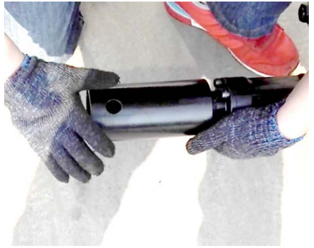
Fig. 2 ) Attach Piling Socket Sleeve by screwing it onto Pile Driver.
