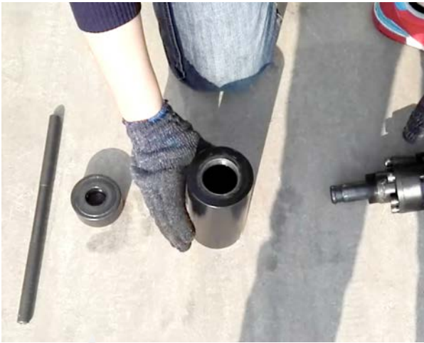
Fig. 1 ) Identify Pile Driver, Piling Socket Sleeves (2 pieces), Inner Pile Head and Socket Pin.
