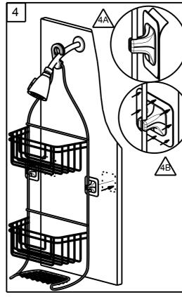
4A) Remove the protective film from the IncrediGrip<sup>™</sup> pads and locate assembly onto mounting surface in desired position. 4B) Using your fingers, partially secure the IncrediGrip<sup>™</sup> pads at each location by pressing the pads firmly into the wall.
