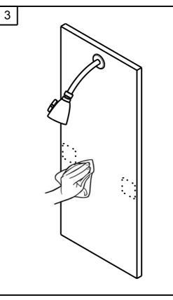
Clean surface areas where IncrediGrip<sup>™</sup> pads will be installed with the provided Isopropyl Rubbing Alcohol pad or Windex® Glass Cleaner and a clean, lint free cloth. Do not use bathroom or other common household cleaners as they may leave a film that prevents pad adhesion or may cause pads to adhere only temporarily to the surface, which could cause the basket to fall and cause injury or property damage.
