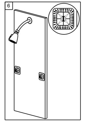
With shower caddy removed, firmly press on IncrediGrip<sup>™</sup> pads and smooth the air bubbles out. Work from mounting post towards the outer edges of the pads. Optimal performance is achieved with removal of all air pockets from under clear pad areas. The failure to remove all air pockets may cause the pads to slip and the basket to fall, causing injury or property damage.
