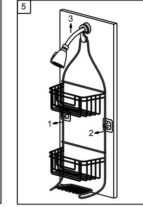
Remove the shower caddy by pulling the left side and then right side of the caddy out of Mounting Posts.
