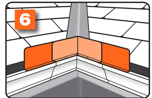
For more protection, cut a SplashShield™ in half, then attach the halves to each side
