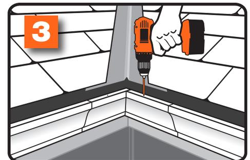
Drill holes as marked with 1/8" drill bit.
