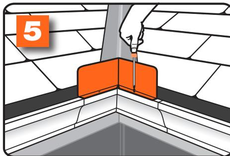
Fasten with aluminum screws on aluminum gutter; stainless steel screws on steel gutter
