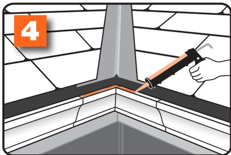
Apply a bead of caulk to the gutter where SplashShield™ will be fastened
