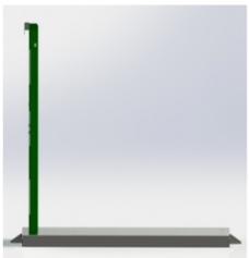
the corresponding slots on one side of the base. Ensure that the tabs are fully engaged (if not fully engaged, the side panel could distort). Gently lift the side panel until vertical. Hit the bottom of the Side Panel with your hand gently on each side, pushing the Side Panel towards the centre of
