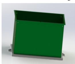
4. Install the Front Panel in the same way as the Rear Panel. Insert the remaining two 1/4" x 3/4" carriage bolts, 1/4" flat washer and 1/4" nut, and tighten.
