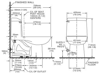
THIS TOILET IS DESIGNED TO ROUGH-IN AT A MINIMUM DIMENSION OF 305MM (12") FROM FINISHED WALL TO C/L OF OUTLET. SUPPLY NOT INCLUDED WITH FIXTURE AND MUST BE ORDERED SEPARATELY.
