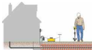
Direct connect to utility lines
