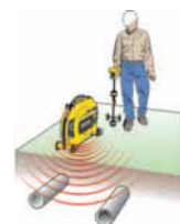
Induce a signal to locate utilities
