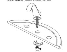
Make connections to water lines. Use 1/2" IPS faucet connections (1) or use the supplied coupling nuts (3) with 3/8" O.D. ball nose risers (2). Use wrenches to tighten connections.Do not overtighten.
