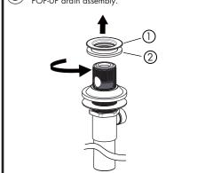
Place the rubber washer (2) to underside of the flange (1). Insert the threaded end of the drain body up through the drain hole and attach flange to the body with the pivot hole (3) pointing to the rear of the sink.
