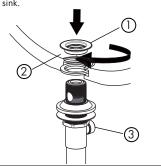
Place one end of spring clip (1) on the end of pivot rod (2) . Insert rod through hole in lift rod strap (3) . Secure with spring clip (1) .
