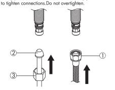
Slide Hot and Cold end valves thru sink mounting Slide Hot and Cold end valves into sink incoming holes. NOTE:Hot side end valve is labeled. Secure end valves with washers and nuts. Hand tighten nuts onto shank. Lock nuts into pisition by tightening screws.
