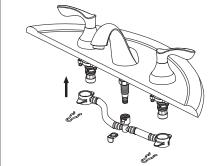
Shut off water supplies.Remove old faucet. Clean sink surface in preparation for new faucet. Place spout thru mounting hole in sink. Secure spout with rubber washer , metal washer and nut.
