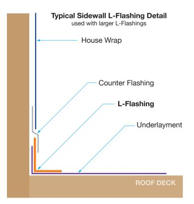
L shaped flashing is a versatile, general use flashing used where a uniform or strengthened finish is needed on a 90 degree surface.
