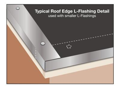
Begin installation along the eaves, starting at a corner and working your way around, overlapping each succeeding piece of drip edge by 2-3 inches.
