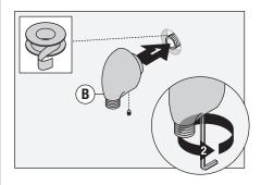
10) Attach large end of hand shower hose (N) to hand shower head (H). Attach small end of hand shower hose (N) and gasket to in-line vacuum breaker (A). Connect in-line vacuum breaker to wall elbow (B). Turn clockwise to tighten.
