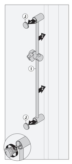
**Notes:** Make sure that 30" slide bar holes and bracket holes are aligned before drilling. Before drilling bottom hole, make sure 30" slide bar is plumb.
