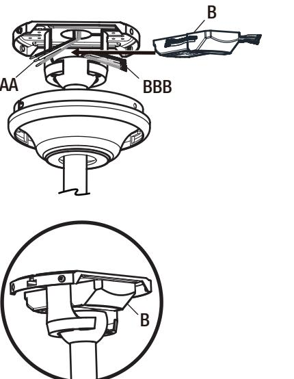
Receiver (B) correctly positioned in the mounting bracket.
