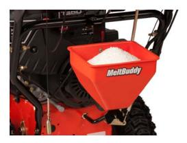
The Ariens MeltBuddy<sup>TM</sup> allows operators to clear snow and spread ice melt in one single pass. The MeltBuddy<sup>TM</sup> has an easy-to-use hand trigger and large capacity hopper which allows the operator to drop ice-melt granules where needed. Available for use on all Sno-Thro units.
