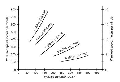
Figure 20: Welding Current vs WFS for ER5356 Aluminum Electrode at a Fixed Stickout
