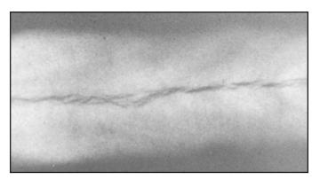
Figure 11: Radiograph Showing Longitudinal Weld Cracking
