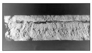
Figure 13: Fracture Surface of a Weld with Incomplete Fusion
