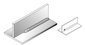
Figure 8: Straight Progression Weld
