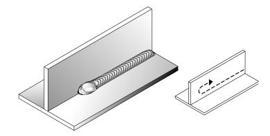
Figure 9: Back Step Technique Weld
