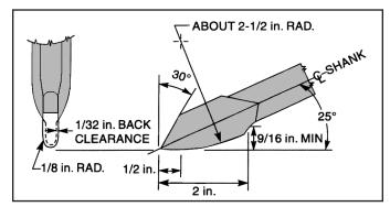
Figure 3: Correct Pneumatic Chisel Geometry for Backgouging Aluminum
