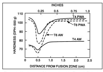
Figure 2: Hardness vs. Distance for 6061-T4 and -T6 in the as-welded and post-weld aged conditions
