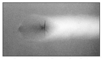
Figure 10: Radiograph Showing a Crater Crack
