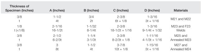
Figure 17: Bend Test Requirements for Wraparound Bend Test Fixture
