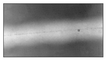
Figure 12: Radiograph Showing Incomplete Penetration
