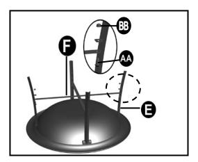
Step 2: Connect each leg (E) to the Fire Bowl (D) using M6 Bolt (AA)
