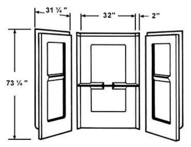
General: Furnish and install as shown on plans, 32" square shower, DURAWALL® Shower Walls Model 732, as manufactured by E.L. Mustee & Sons, Inc. Shall be 3-piece, molded fiberglass wall with minimum thickness of 25 mils and mounts direct-to-studwalls. Includes center panel with molded-in shelves, built-in towel bar and two side panels with molded-in shelf. Self aligning panels interlock using a tongue-and-grove connection. Shall meet ANSI Specification Z 124.2A—1990. Color\_\_\_\_ (White, Bone).
