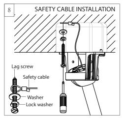
For Canadian installation and for USA fan and light kit combinations over 35 lbs, in both flush and downrod modes the safety cable must be installed into the house structure beams using 3" lag screws, washers and lock washers provided. Make sure that when the safety cable is fully extended the lead wires are longer than the cable and no stress is placed on the lead wires.
