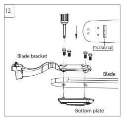
Align the holes of blade bracket, blade and the bottom plate of blade bracket. Install blade bracket with blade by 4 blade screws provided. Tighten screws securely. Repeat this process for remaining blades. **Note**: Make sure the side with a label "This side up" is installed upward.
