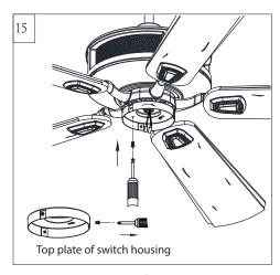
Remove 3 set screws from top plate. Keep screws.
