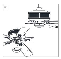
Attach switch housing onto top plate, aligning the holes and reinstall the 3 set screws removed in step 15 and tighten all screws securely.
