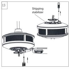
Remove shipping stabilizers from motor assembly.
