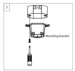
Use metal outlet box suitable for fan support and use only the screws provided with the outlet box (must support 35 lbs). Before attaching fan to outlet box, ensure the outlet box is securely fastened by at least two points to a structural ceiling member (a loose box will cause the fan to wobble). Remove the two outlet box screws provided with the box, aligning the holes of the mounting bracket with the holes of the outlet box. Reinstall the 2 outlet box screws securely.
