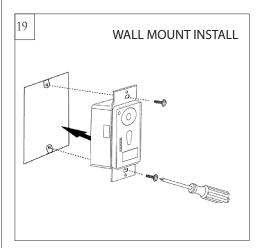
Install wall control unit to outlet box using machine screws provided.
