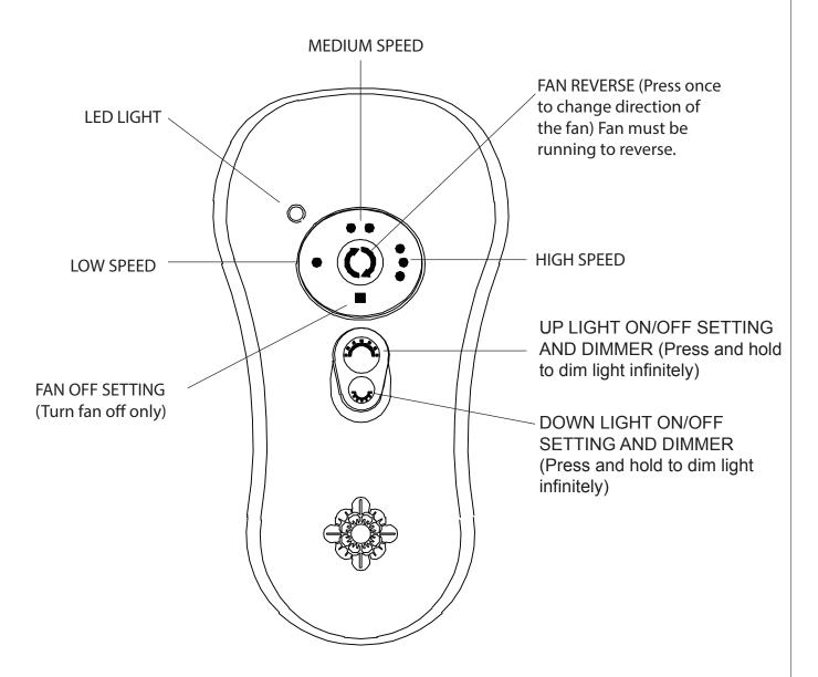
FAN SPEED: Depress "1 dot" for low speed, "2 dots" for medium or "3 dots" for high. To turn fan off press square".
