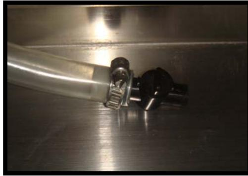
B. Flow Control Valve (Inside Reservoir)
