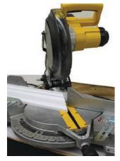
STEP 2 – To complete the miter, rotate the table angle gage to the opposite  $45^{\circ}$  angle. And insert the mating piece of trim in the left hand position. Then proceed with the cut. See photo #2 to the right.
