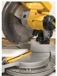
STEP 1 - Place the casing on the saw in the LH horizontal position with the "outside of the trim" against the fence. Rotate the table angle adjustment to the "left" 45° setting and make the initial cut. See photo to the right.
