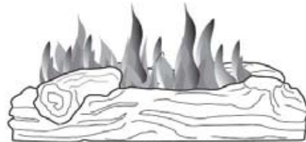
Figure 22 - Incorrect Burner Flame Pattern
