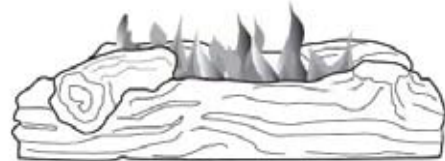
Figure 21 - Correct Burner Flame Pattern
