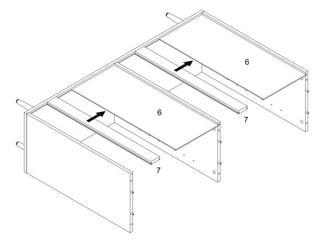
Slide part (7) into grooves and attach to part (6) as per diagram.
