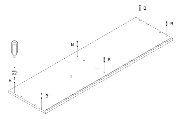
Secure cam bolt (B) to part (1) with Philips head screwdriver.
