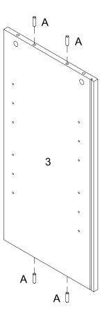
Insert wooden dowel (A) into part (5, 4, 3) as per diagram.
