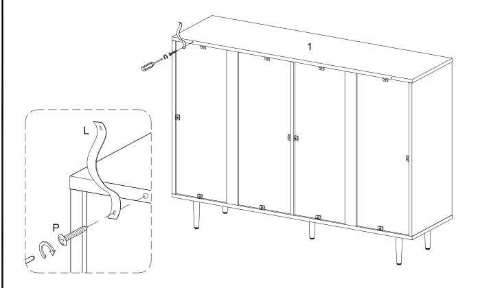
Attach plastic strap (L) to back of part (1) using screw (P) with Philips head screwdriver.
