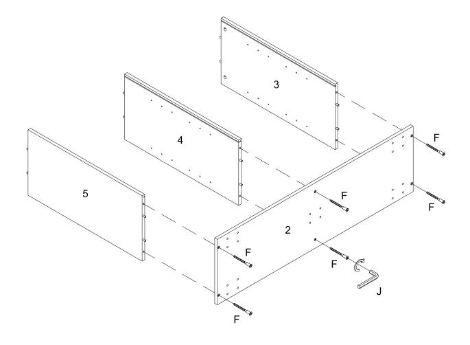
Attach part (2) to part (5, 4, 3) using screw (F) with hex key (J) as per diagram.
