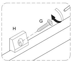
Secure plastic wedge (H) to back panel using screw (G) with Philips head screwdriver as per diagram.
