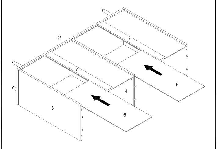
Slide part (6) into grooves of part (7, 4, 3) as per diagram.
