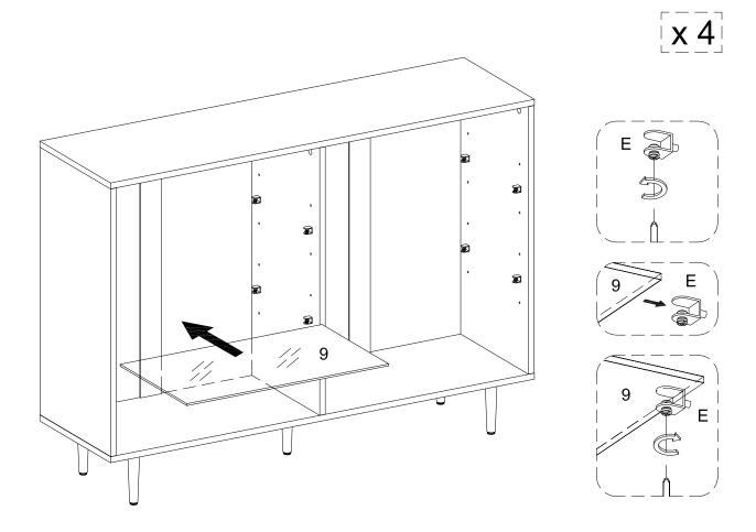
Loosen screw of glass holder (E), place and secure part (9) to glass holder (E) with Philips head screwdriver as per diagram.
