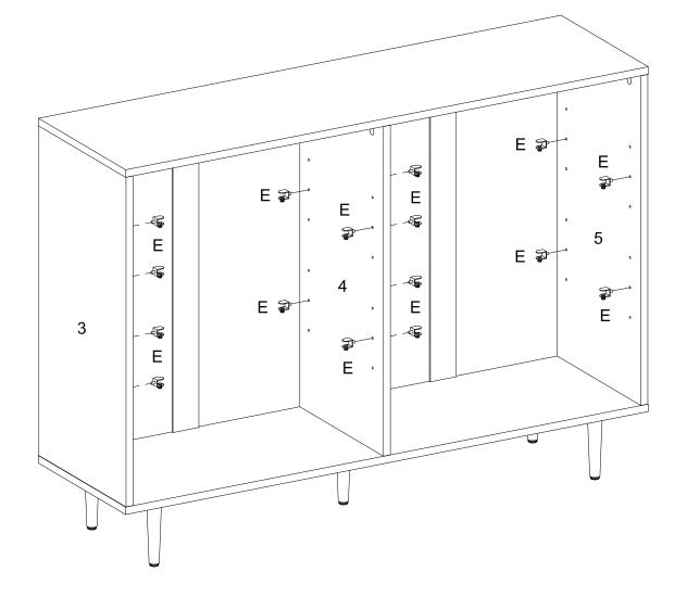
Insert glass holder (E) into part (3, 4, 5) as per diagram.
