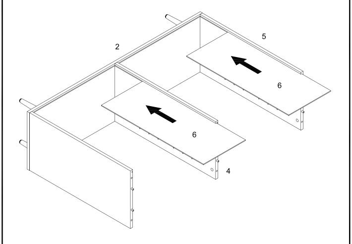
Slide part (6) into grooves of part (4, 5) as per diagram.
