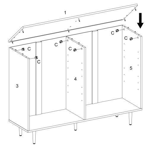
Attach part (1) to part (3, 4, 5) using cam lock (C) with Philips head screwdriver.
