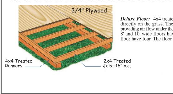
**Deluxe Floor:** 4x4 treated runners can be installed directly on the grass. The runners elevate the floor providing air flow under the floor eliminating moisture. 8' and 10' wide floors have three runners, 12' wide floor have four. The floor covering is 3/4" plywood.
