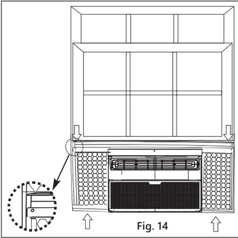
In order to minimize air leaks between the room air conditioner and the window opening, trim the weather stripping to the proper length, peel off the protective backing and plug any gaps if needed (Fig. 14).
