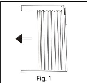
A. Place unit on floor, a bench or a table. Hold the Accordion Panel in one hand and gently pull back the center to free the open end. See Fig. 1.
