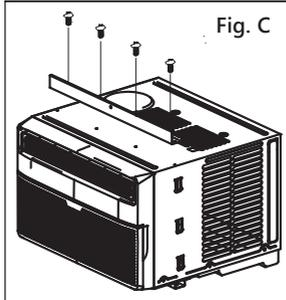
C. Align the hole in the top rail with those in the top of the unit as shown in Fig. B.
