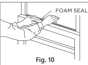
D. Cut Window sash seal foam and insert it in the space between the upper and lower sashes (Fig. 10).
