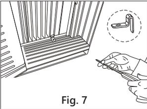
A. Place the frame lock between the frame extensions and the window sill as shown (Fig. 7).
