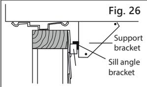
Refer to Step 5 of Window Mounting for assembly of support brackets. A wooden strip nailed to the outside wall should be used in conjunction with sill support angle brackets.
