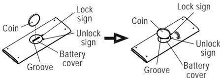
**Step 3:** Replace the battery cover, making sure the battery cover groove is aligned with the “unlock” sign. Insert a coin vertically in the groove and press it gently, then rotate 45° counter clockwise, making sure the groove is aligned with the “lock” sign as shown below.
