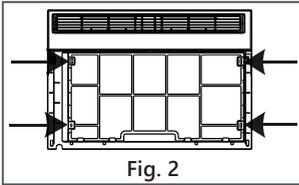
3. Locate the four front screws and remove. These screws will be needed to re-install the front panel (see Fig. 2).
