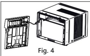
6. Disconnect the connector plug of the display panel from the unit and place front panel to one side (see Fig. 4).
