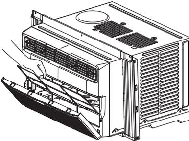
The air filter should be checked at least once a month to see if cleaning is necessary. Trapped particles in the filter can build up and cause an accumulation of frost on the cooling coils.
