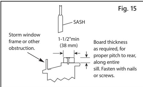
Add wood as shown in Fig. 15, or remove storm window before air conditioner is installed.
