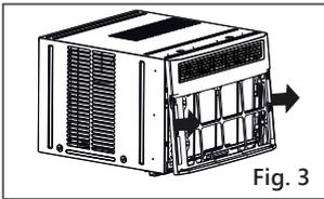
4. Push metal cabinet side to release plastic tabs on each side of front panel (see Fig. 3).
