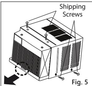
7. Remove shipping screws from top of unit and also on the side by the base if installed (see Fig. 5).
