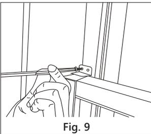
C. To secure lower sash in place, attach right angle sash lock with 3/4" (19 mm) or 1/2" (12.7 mm) screw as shown (Fig. 9).
