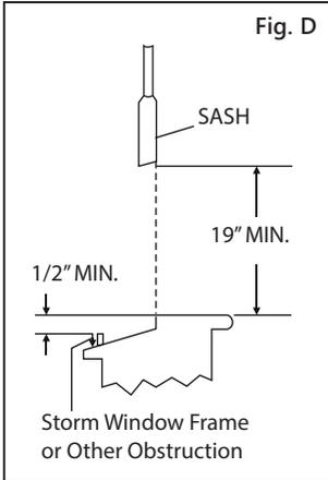
1. Check window opening size - the mounting parts furnished with this air conditioner are made to install in a wooden sill double-hung window. The standard parts are for window dimensions listed above. Open sash to a minimum of 19" (483 mm). See Fig. D.
