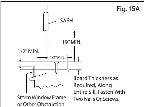
Check your storm windows - if your storm window frame does not allow the clearance required, correct by adding a piece of wood as shown in Fig. 15A, or by removing storm window while room air conditioner is being installed.
