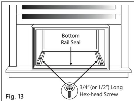
5. Add bottom rail seal over screws to window sill. (Fig. 13).
