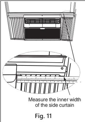
In order to minimize air leaks and ensure optimal insulation, it is necessary to install the included R1 hardware to the side curtain. Follow the instructions below.
