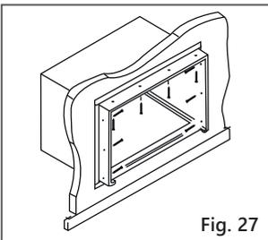
5. Screw or nail cabinet wooden frame using shims if frame is oversized, to minimize distortion. See Fig. 27. Remember to maintain proper slop as described in Step 3.
