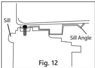
3. Shift cabinet left or right as needed to line up center of cabinet on center line marked on sill.
