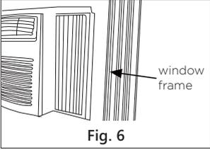
B. Extend the side panels out against the window frame (Fig. 6).
