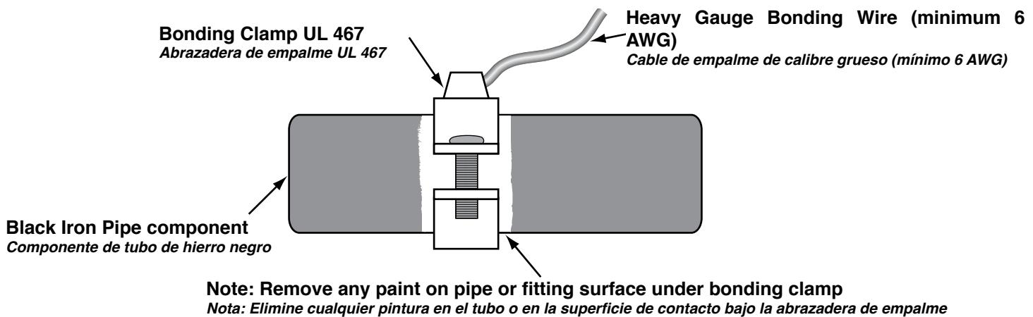
**NOTE: DO NOT connect bonding clamp directly onto HOME-FLEX® tubing**
