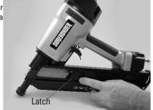
To remove fasteners: Depress the latch and release the feed #\$hoe and slide it forward. Remove fasteners from the tool.
