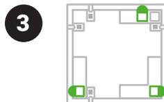
Attach 3 pieces of mounting tape to the back of each Light Square, spaced evenly.
