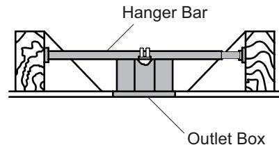
To hang your fan where there is an existing fixture but no ceiling joist, you may need an installation hanger bar as shown above (available at any Home Depot store).
