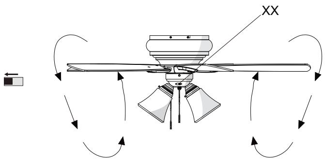
**Warm weather - (Forward)** A downward airflow creates a cooling effect. This allows you to set your air conditioner on a warmer setting without affecting your comfort.
