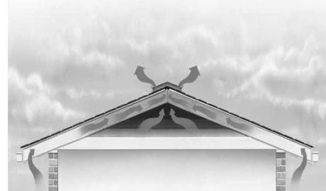
To calculate the minimum amount of total ventilation required, use either the 1/300 or 1/150 ratio. On the inside, the actual calculations have been made for your convenience. Use the 1/300 ratio if you have proper distribution of soffit and ridge vents or if a vapor retarder is present. Use the 1/150 ratio if proper distribution of soffit and ridge vents cannot be achieved and a vapor retarder is not present.
