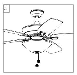
Install fan and light kit pull chains to preassembled pull chains on fan. Pull chains provided.
