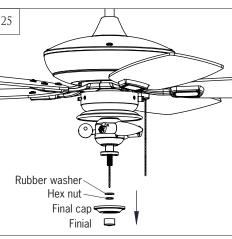
Remove finial, final cap, hex nut and rubber washer from light fixture. Keep the parts.
