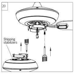
Remove shipping stabilizers from motor assembly.
