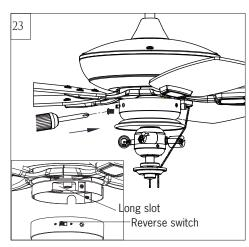
Align the long slot on top plate with the reverse switch on light fixture, and then install the light kit onto the top plate with the 3 set screws removed in step 21 and tighten all screws securely.
