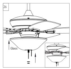
Raise glass in order to guide pull chains through appropriate holes in glass, aligning threaded rod on light fixture with hole in middle of the glass and push up gently allowing threaded rod to come through hole. (**Note**: Be sure pull chain for fan operation does not rub against bulb during operation).
