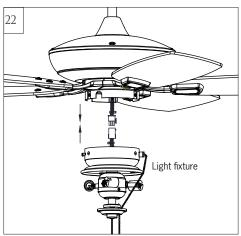
Connect the plug from fan with the plug from light fixture. Be sure plugs connection clasped together completely.
