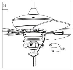
Install 3 x 60 watt candelabra base bulbs, Bulbs included. **WARNING**: Over lamping the fan will result in the fan lights shutting down until the proper wattage of bulbs are installed. Reset the lights by turning off the wall switch, breaker,or by remote. Replace bulbs with the correct wattage bulbs, turn the power on.
