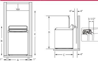
To ensure sufficient clearance for water lines and airflow, allow minimum clearances of at least 1 in. (2.5 cm) at the sides and 4 in. (10 cm) behind the unit. Be sure to allow for wall, door, or floor moldings that may increase the required clearances.
